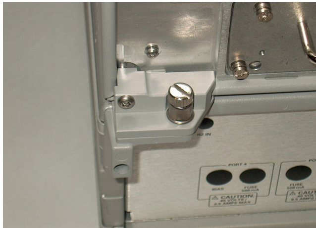
Figure 10 Locking Feet Screws
