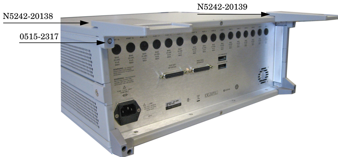
Figure 14 Install Locking Feet on Test Set
