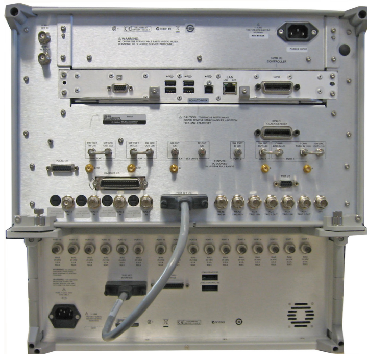
Figure 18 Test Set I/O Cable Connection
