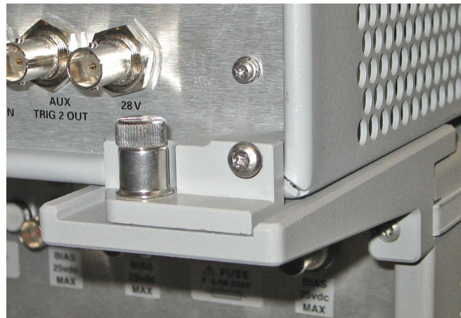
Figure 16 Locking Feet Screws
